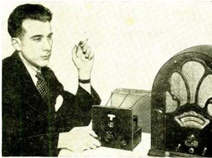
The author adjusting the D.C. converter while bringing in a distant short-wave station.
