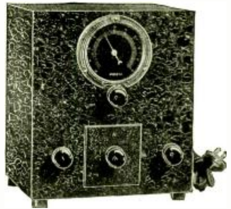
Above—Front view of the new Postal 2-stage R.F. Booster which can be used ahead of any receiver. Below—Wiring diagram of the Booster.
