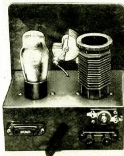
This picture shows a rear view of this unusual "1-tube" receiver—the Duo-Amplidyne, developed especially and exclusively for SHORT WAVE CRAFT readers by the author.
