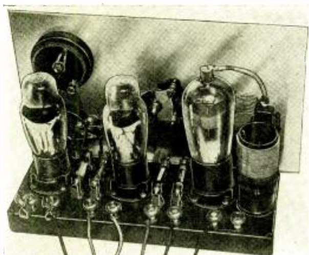
Rear view of the "Jiffy 3" which features "simplified" wiring.
